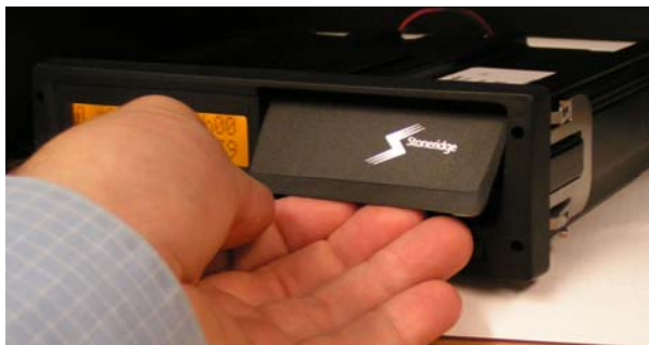
3. Hold the fascia at the bottom where it is tilting outwards.
