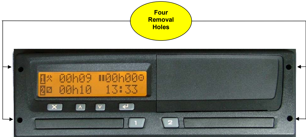
Figure 15 Position of VU Removal Holes
