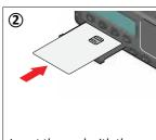
Insert the card with the chip facing upwards.
