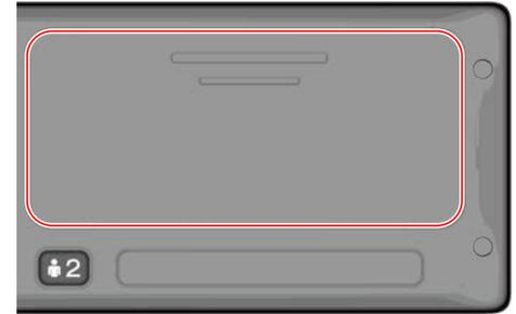
Behind the printer panel there is a printer containing a paper cassette with a paper roll. The printer is used e.g. to make printed records of information stored in the tachograph. The printed paper will come out from a small opening at the bottom of the printer panel.
