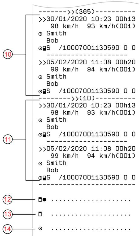
10. Five most serious overspeeding over the last 365 days. Date time and duration. Max and average speed. Driver and drivers card identification.
